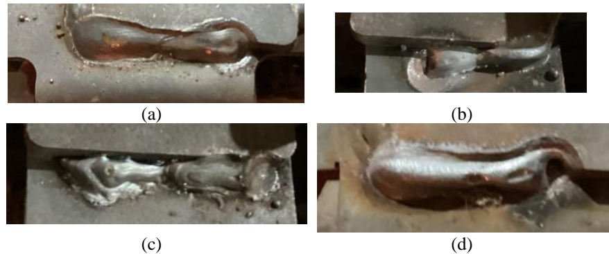
Fig. 10. Examples of weld seams belonging to the four categories. (a) Good, (b) Robot, (c) Human, and (d) Scrap.
